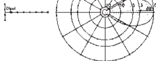
Vertical Radiation Pattern E Plane
