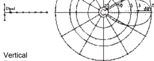
Horizontal Radiation Pattern H Plane
