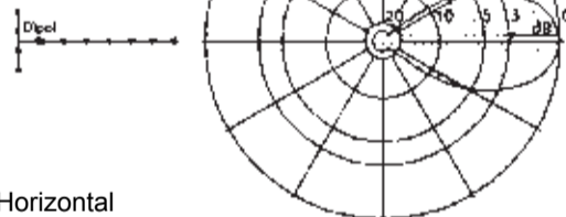
Vertical Radiation Pattern E Plane
